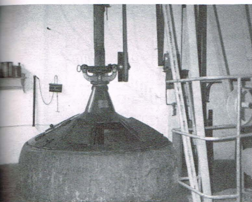
The boiling kettle at the Cantillon brewery in Brussels. The belt and pulley above the kettle drive a dasher by the steam coils inside. On the far right of the frame is a belt-driven
